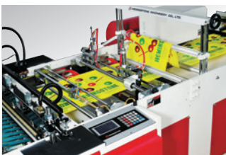
Photocell Control and Pre-sealing Station
