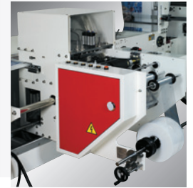
Patch Welding Unit
